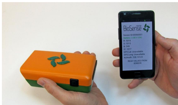
Figure 12: Plant-O-Meter and specifically designed smartphone application.
