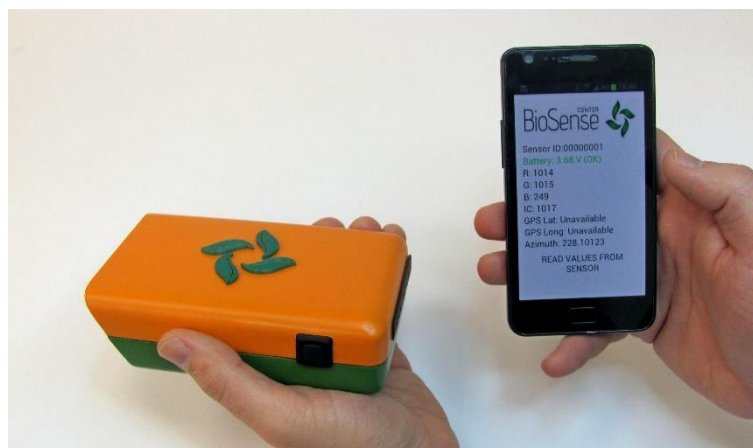
Figure 12: Plant-O-Meter and specifically designed smartphone application.
