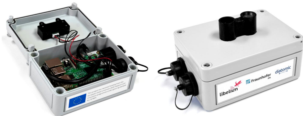
Figure 36: Libelium platform in housing, LIDAR sensor protruding on the top (facing down in final setup)
