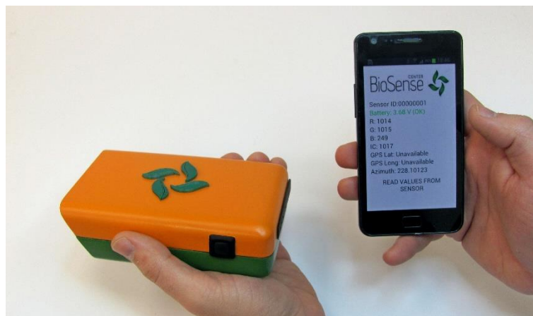
Figure 12: Plant-O-Meter and specifically designed smartphone application.
